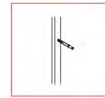
1 Joist span is 600 mm. Fix the joist every meter with expansion screw
